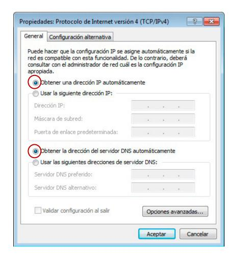
At this new screen *Obtain an IP address automatically* and *obtain DNS server address automatically* options should be selected.
